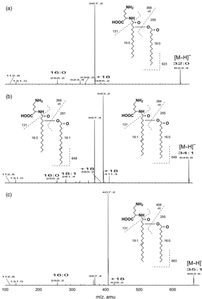
**Fig. 4.** Negative-ion electrospray MS/MS spectra of the three dominant molecular ion signals from OLs. (a) Major fragments of the 623.4  $m/z$  molecular ion corresponding to a 32:0 OL; (b) major fragments of the 649.6  $m/z$  molecular ion corresponding to a 34:1 OL; and (c) major fragments of the 663.6  $m/z$  molecular ion corresponding to a 35:1 OL. The position of any unsaturation is currently unknown.
