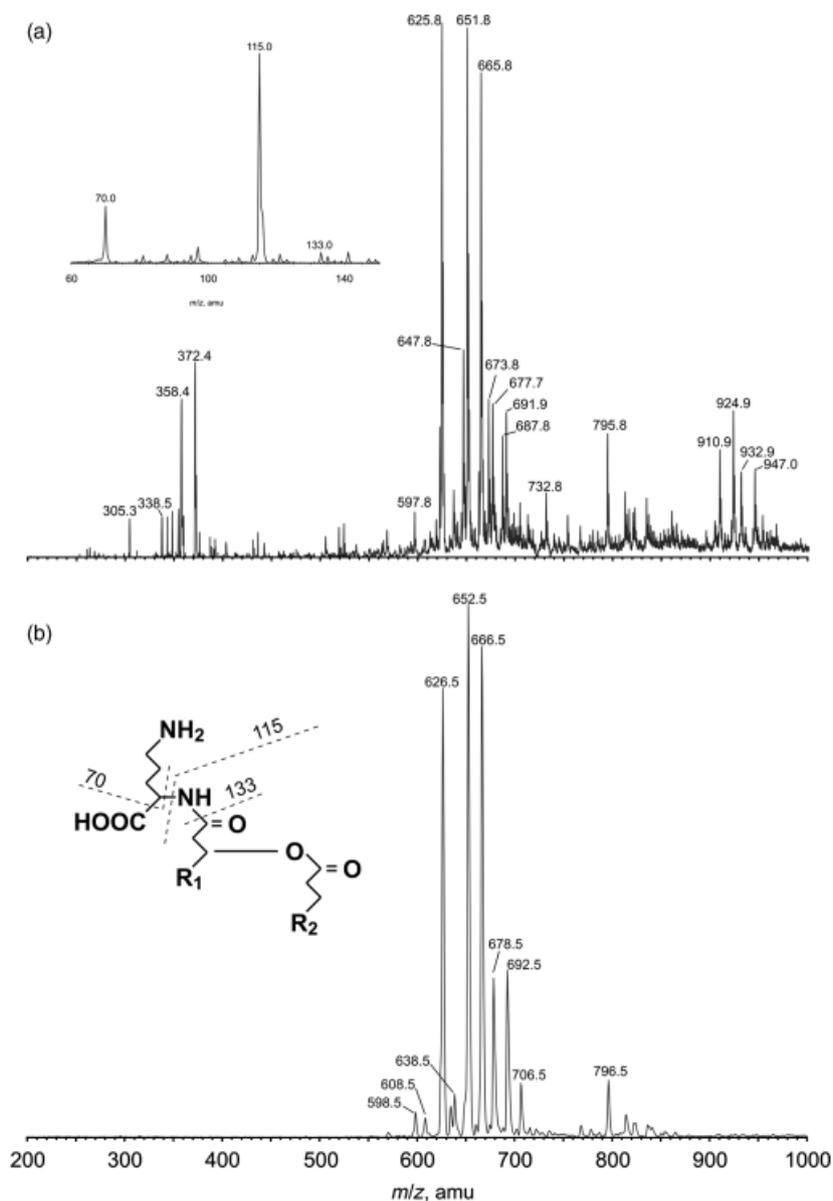
**Fig. 3.** Positive-ion mode electrospray mass spectra of the suspected OLs purified from *Pseudomonas aeruginosa* grown under low-phosphate conditions. (a) Positive-ion spectrum of OL fraction. (b) Positive-ion precursor spectrum showing molecular masses for lipids containing a 115  $m/z$  fragment ion. The inset structure shows the formation of the 115/116  $m/z$  ornithine ion, also reported for ornithine-lipids found in *Rhodobacter capsulatus* (Aygun-Sunar *et al.*, 2006).
