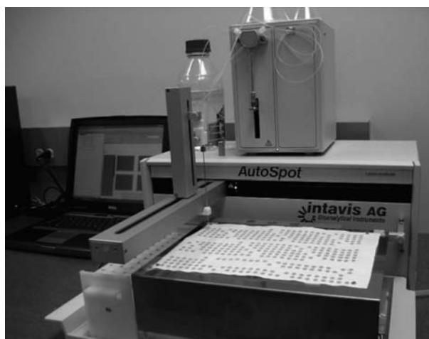
Fig. 5.2. Semi-automated synthesis of large spots using AutoSpot robot (INTAVIS).
