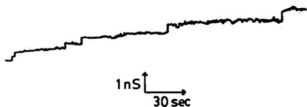
FIG. 5. Conductance increases after addition of 0.6 ng of purified porin protein F from *E. coli* JF733(pHN4) per ml to the aqueous 1 M KCl solutions bathing a lipid bilayer membrane. The applied voltage was 50 mV. The chart recorder tracing started on the left after the membrane had turned black. Each conductance step involved incorporation of a single porin channel into the membrane.
