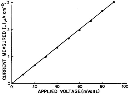
FIG. 3. Relationship between the mean current through single channels ( $I_m$ ), averaged for a large number of conductivity increases ( $n > 100$ ), and the voltage applied across the bilayer membrane. Otherwise, conditions were as described in the legend to Fig. 2.
