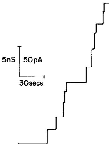
FIG. 4. Stepwise increase of the membrane current after addition of purified protein K to a final concentration of  $5 \times 10^{-11}$  M ( $6 \text{ pg} \cdot \text{ml}^{-1}$ ) into the aqueous phase containing 1.0 M KCl; temperature, 25°C. The membrane was formed from a 1% (wt/vol) solution of oxidized cholesterol in *n*-decane. The applied voltage was 10 mV. The record begins at the left; usually only upward directed current increases were observed.
