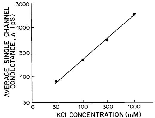
FIG. 6. Average single-channel conductance ( $\bar{\Lambda}$ ) as a function of KCl concentration in the aqueous phase; temperature, 25°C. Membranes were formed from 1% (wt/vol) oxidized cholesterol in *n*-decane. Protein K ( $5 \times 10^{-12}$  M) was added to the aqueous phase, and conductance increments were averaged for 74 to 158 individual events.
