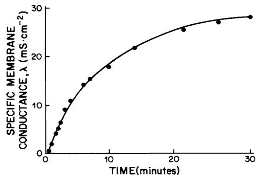
FIG. 2. Time course of increase of macroscopic conductance caused by the addition of 42  $\mu$ g of purified protein K per ml to the aqueous solution bathing a lipid bilayer membrane. Experiments were performed at 25°C, using membranes made from 1% oxidized cholesterol in *n*-decane with 1.0 M KCl as the bathing solution and an applied voltage of 10 mV.
